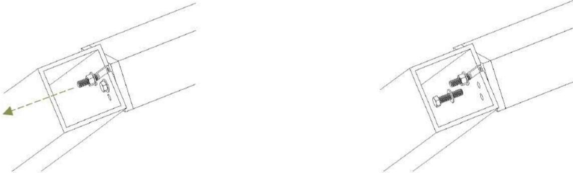
*Hold the track supporting beam and slowly release the nut on the protruding thread until rotation is possible*
