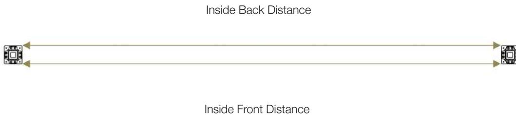
Ensure the back (or front) of the bases are co-linear by dropping a chalk line.
