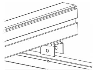
**Step 3:** Hold the wing and release the G-clip.
